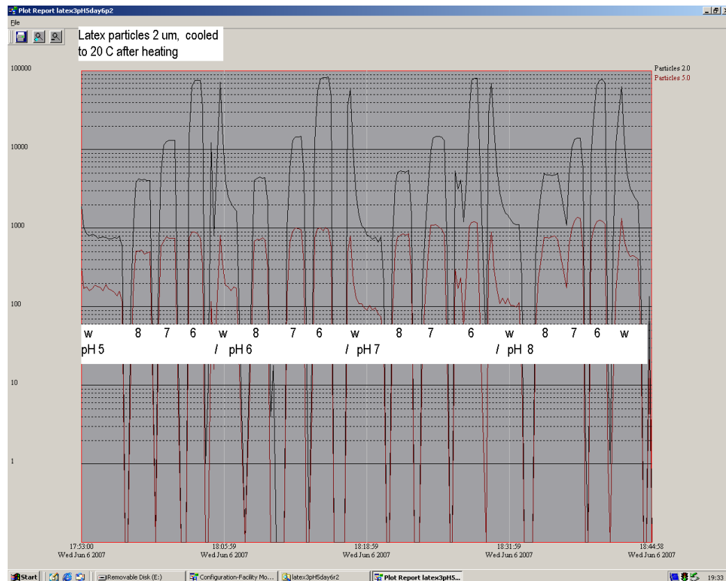
Figure 2 Latex particle size 2 \mu\text{m} cooled to temp 20°C after heating up to 40°. Read by channel size 2, 5 \mu\text{m}
