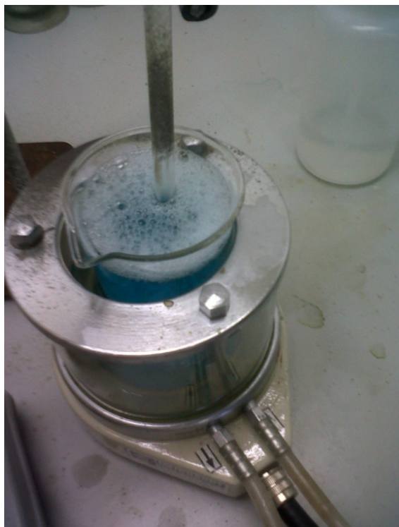
Figure (17) Experimental set up for air bubbling experiments
