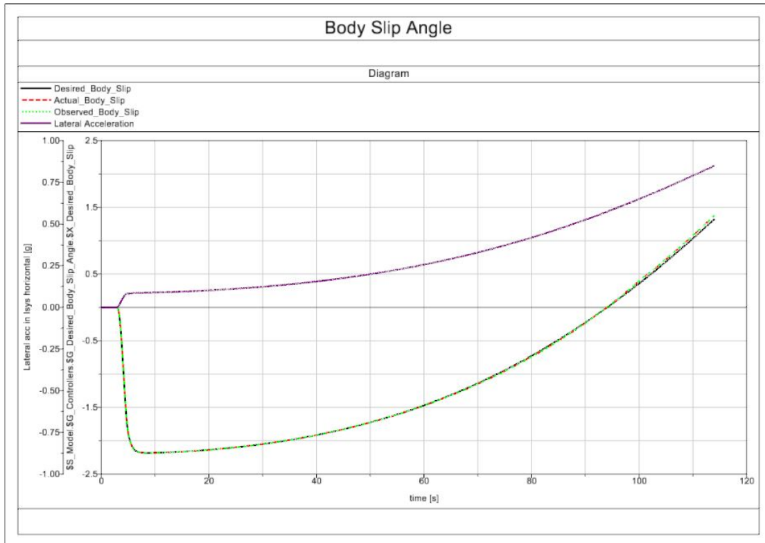
Figure 55 Body Slip Angle and Lateral Acceleration Results with Varying Cornering Stiffness Included, and ESC System Enabled from Constant Radius Loadcase
