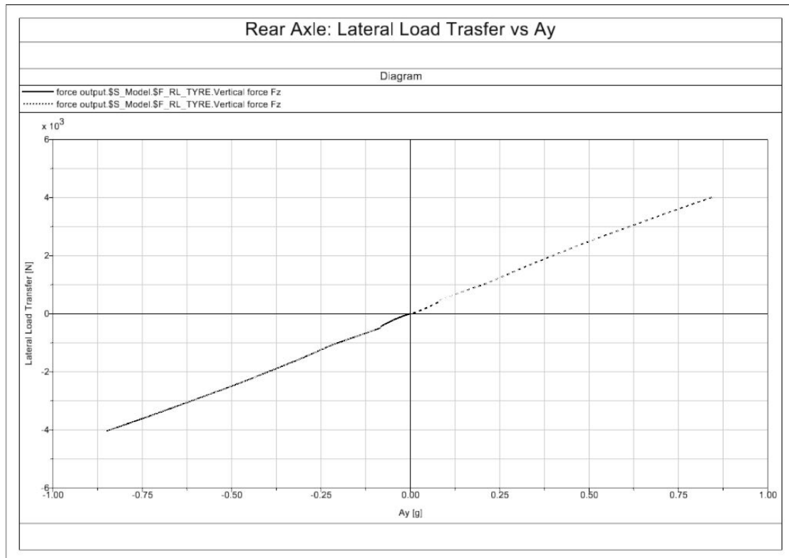
Figure 45 Rear Axles: Lateral Load Transfer vs. Lateral Acceleration (g) From Constant Radius Loadcase
