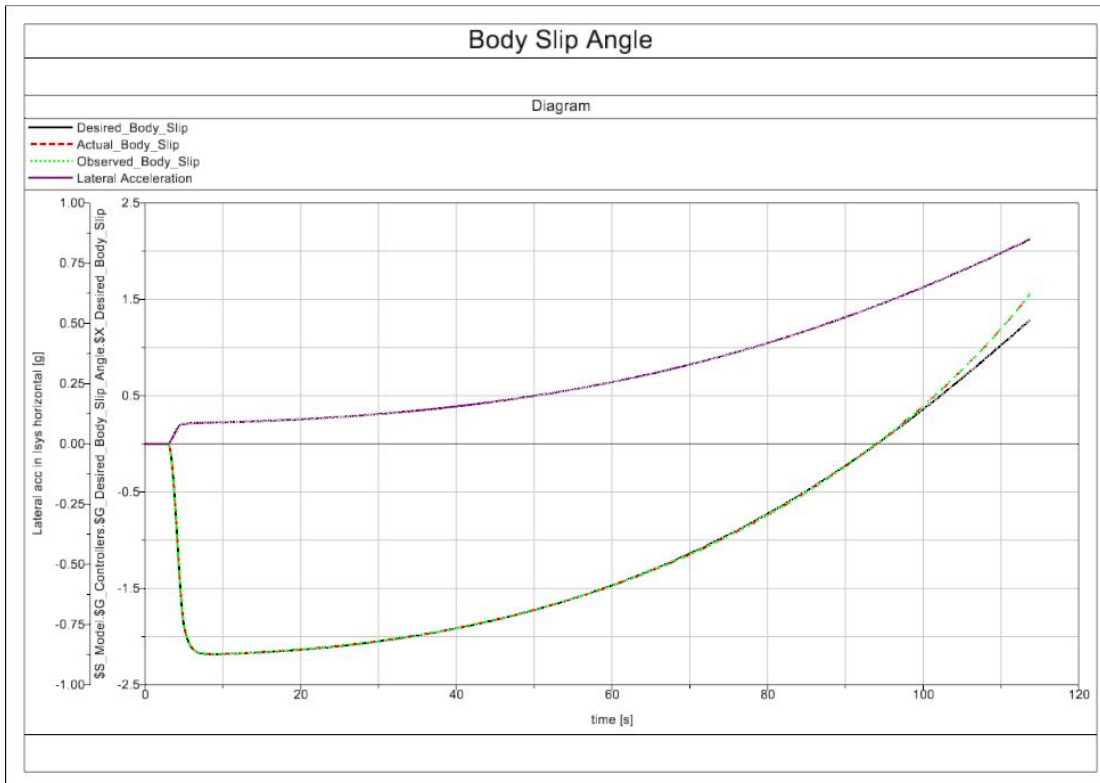
Figure 54 Body Slip Angle and Lateral Acceleration Results with Varying Cornering Stiffness included, from the Constant Radius Loadcase
