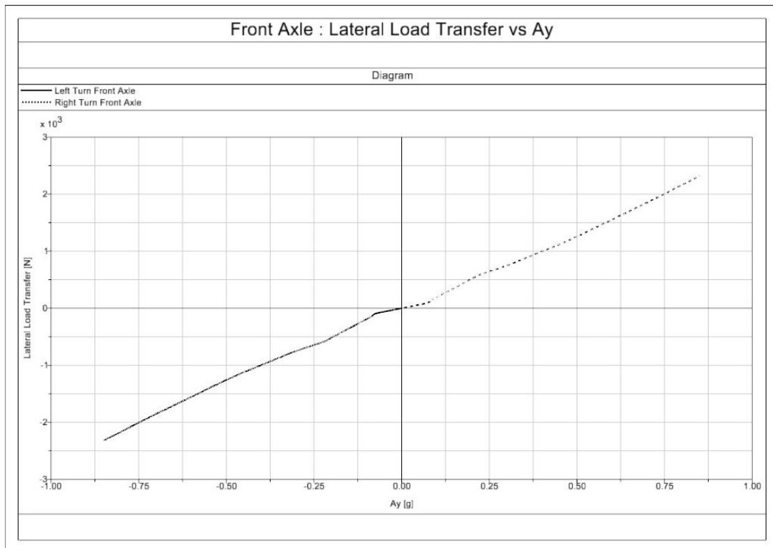
Figure 44 Front Axle: Lateral Load Transfer vs. Lateral Acceleration (g) From Constant Radius Loadcase
