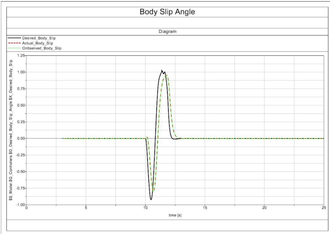
Figure 56 Desired Body Slip Angle, Actual Body Slip Angle and Observed Body Slip Angle for the Sine with Dwell Loadcase at Amplitude "A"
