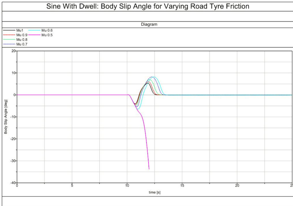
Figure 62 Sine with Dwell: Body Slip Angle for Varying Road Tyre Friction
