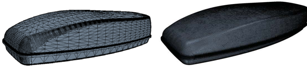
Figure 20: Surface of roof box before and after surface remesher
