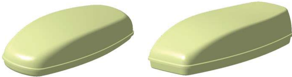
Figure 18: Comparing the shapes of modified box with original roof box
