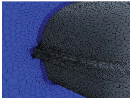
Figure 22: Prism layer and polyhedral meshing
