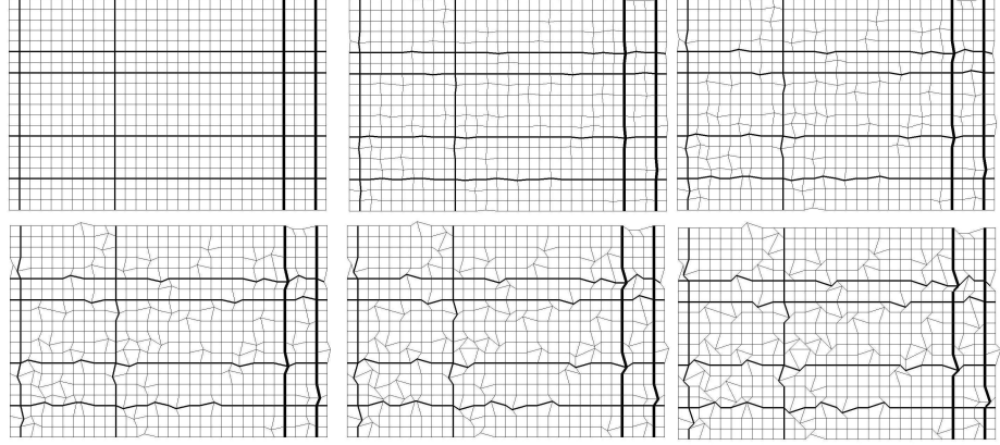
Figure 3.1: Example outputs of the grid based road network generation algorithm with different values of vertex displacement parameter (from 0.0 in the top left to 1.0 in bottom right).
