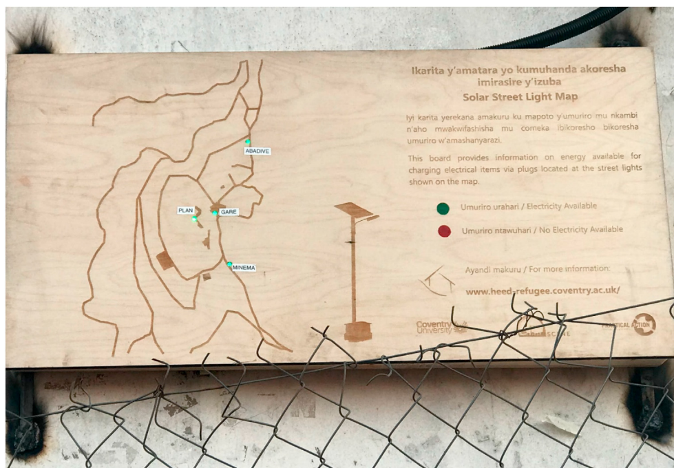
Fig. 4. Advanced streetlights socket energy availability interface board, Gihembe, Rwanda: displayed in a public space in the camp, with high traffic and visibility.
