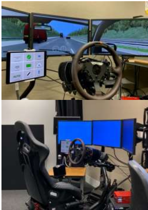
Figure 1 WMG 3x3 Development Simulator, with an iPad positioned as a surrogate center console display
