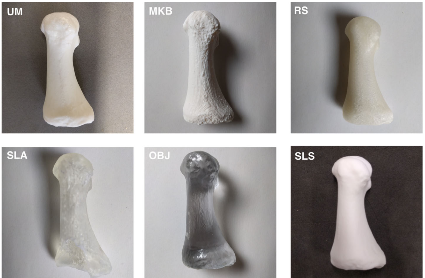
FIG. 3—Lateral views of six 3D printed replica metatarsals. [Color figure can be viewed at wileyonlinelibrary.com ]
