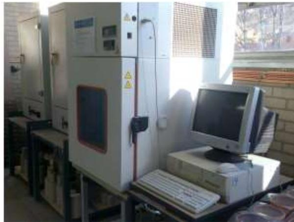
**Fig. 4.15 Environmental chamber for freeze-thaw resistance test**
