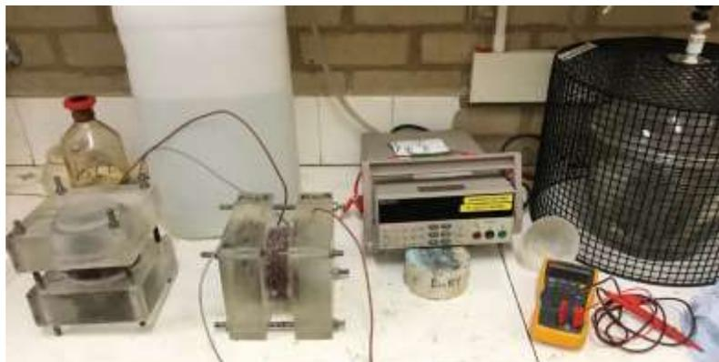
**Fig. 4.17 RCPT test for the GC/Na-R concrete**
