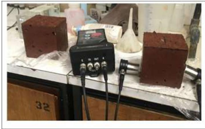
**Fig. 4.12 UPV test for GPC/Na-R concrete**
