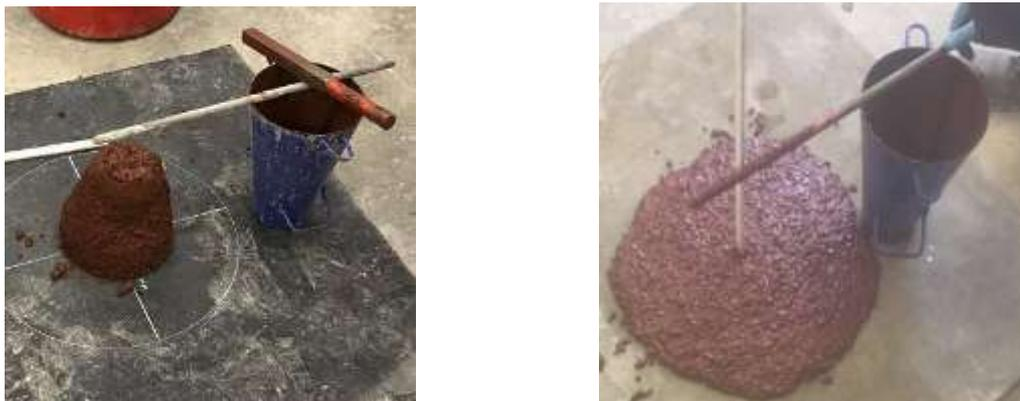
**Fig. 4.7 Slump measurement for the geopolymer concrete mixes**
