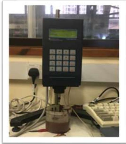
**Fig. 4.9 Rheology test for the geopolymer grout**
