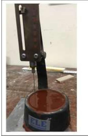
**Fig. 4.10** Setting time test for the calcined clay geopolymer grout
