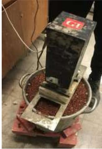
**Fig. 4.8 Rheology test for the calcined clay geopolymer concrete**
