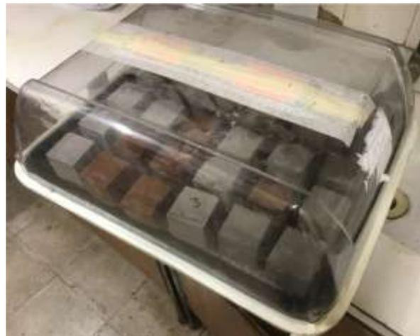
**Fig. 4.6** Compaction and sealed curing of semi-dried samples
