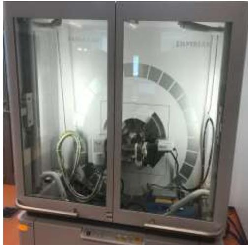
**Fig. 4.19 XRD set-up for the various mortar and concrete samples**
