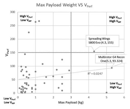
Figure 5. Max payload VS performance variable for a range of multicopter UAV models.
