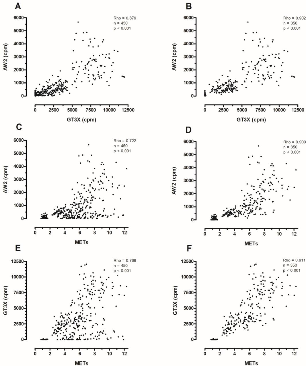
**Figure 2.** Correlations between counts measured by the AW2 and GT3X accelerometers (**A, B**), AW2 counts and task MET (**C, D**) and GT3X counts and task MET (**E, F**). The left panel includes all tasks (**A, C, E**) while the cycling tasks are omitted from the right panel graphs (**B, D, F**). cpm: counts per minute; MET: metabolic equivalents. Correlations were determined using Spearman's rho test.
