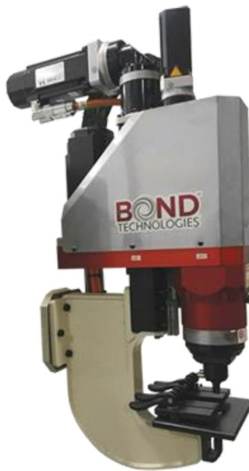
Figure 2.28 - Bond technologies RFSSW system (Bond technologies 2018)
