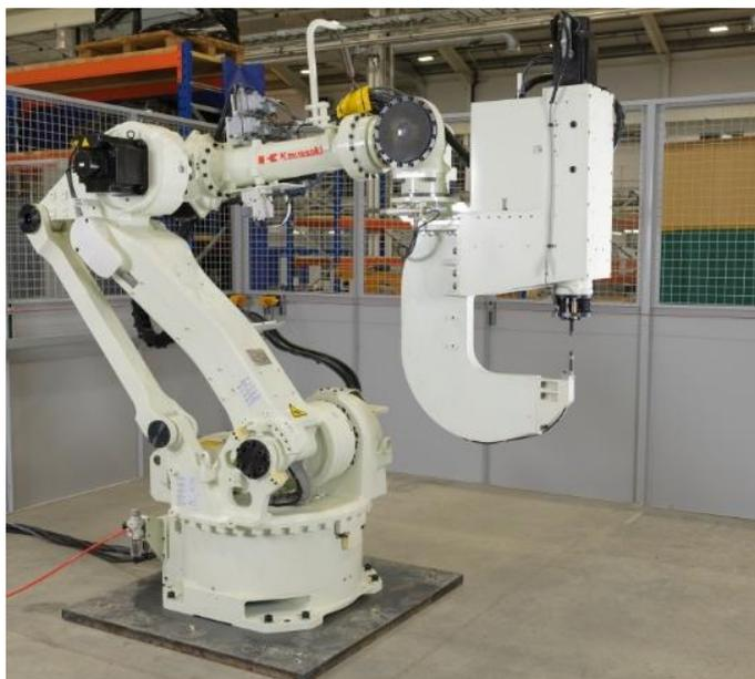
Figure 3.1 - TWI's FW-35 KHI RFSSW system.
