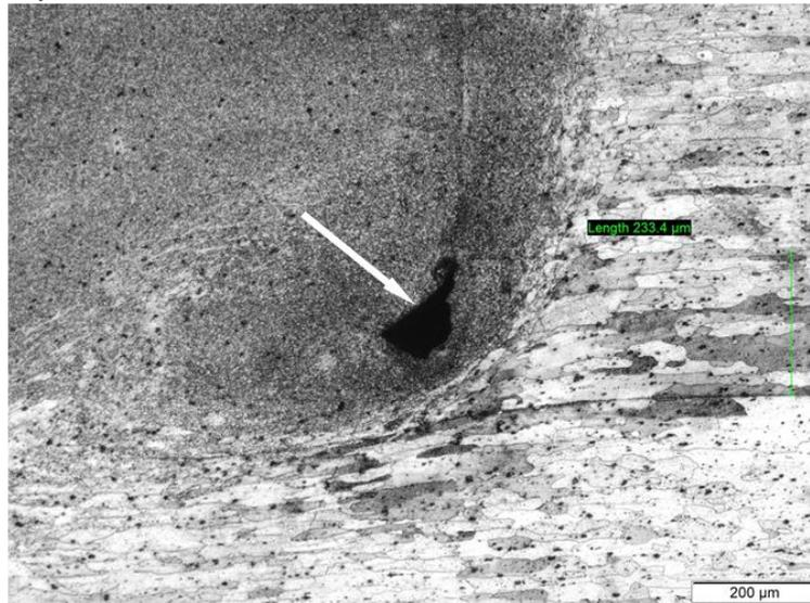
Figure 3.38 - Internal defects on the cross-section of RFSSW AA2024-T3 condition W1 (RS = 1000 rev/min; PD = 2.0 mm).
