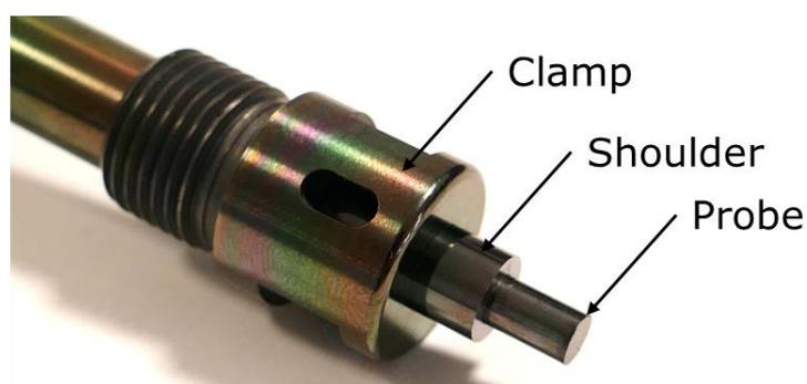
Figure 3.2 - KHI RFSSW tool components.
