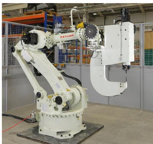
Figure 2.27 - KHI RFSSW system (Courtesy of TWI, Ltd).
