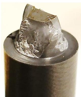
**Figure 4.4 - Fracture surface of a  $\text{Si}_3\text{N}_4$  tool after 92 plunges.**
