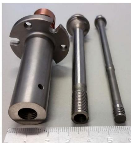
Figure 2.11 - RFSSW tool with a threaded shoulder from H&W (Nasiri et al. 2018).
