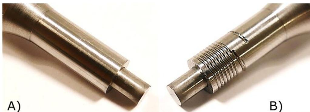
Figure 5.2 - Shoulder and probe design for A) Tool 2 and B) Tool 3 RFSSW tool sets.
