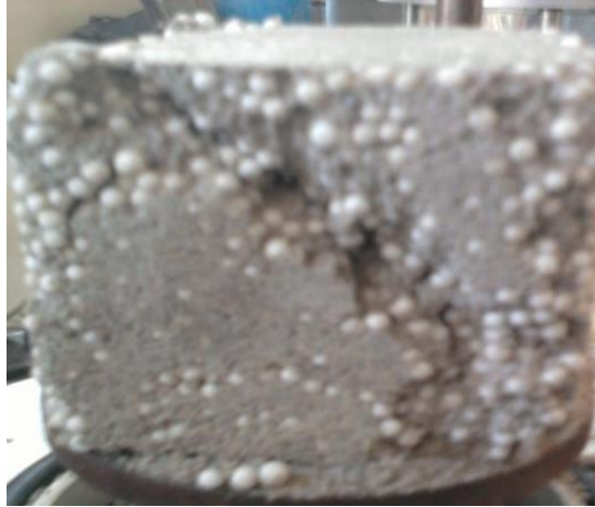
Fig. 7 Failure shape of the cube after unconfined compression test
