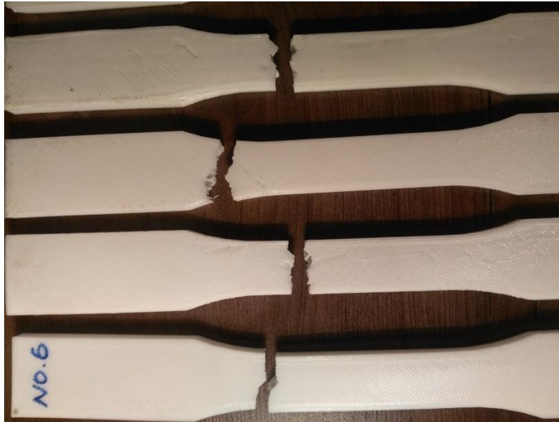
Figure. 3. fracture of the specimen after tensile test
