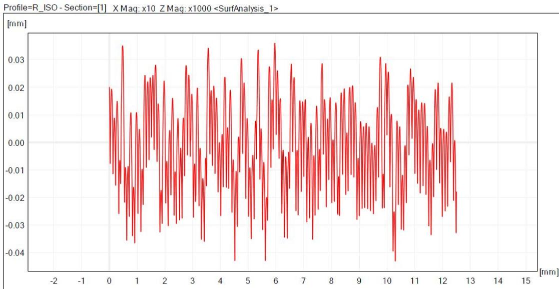
Figure A3. 2: Surface roughness profile on the chosen patch from the leading edge of the printed aerofoil
