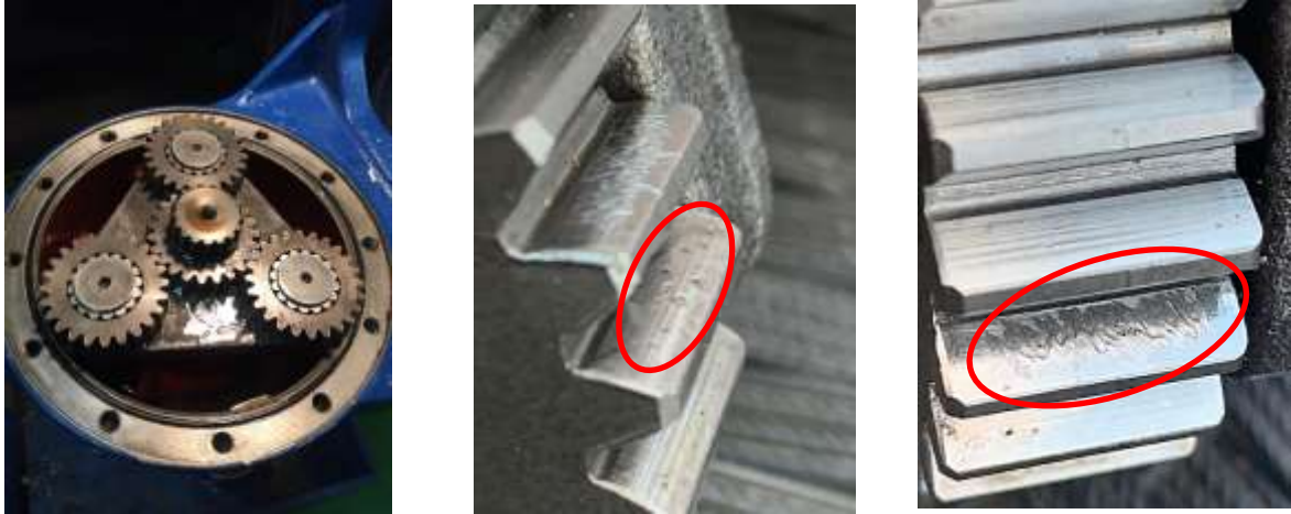
Fig. 10 Dismantled gearbox (left), natural pitting (middle) and induced pitting on the planet tooth (right)
