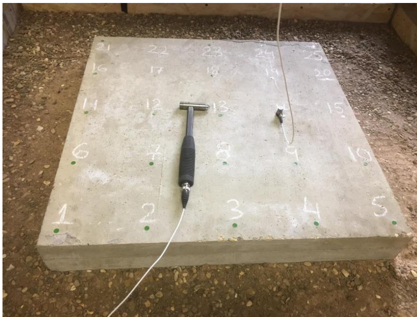
Figure 5-31: Test 06. Two slabs, 'fully-bonded' supported on subgrade.
