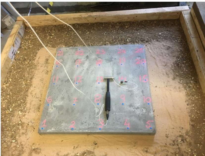
Figure 5-24: Test 03. Single ‘robust’ concrete slab, supported on subgrade.
