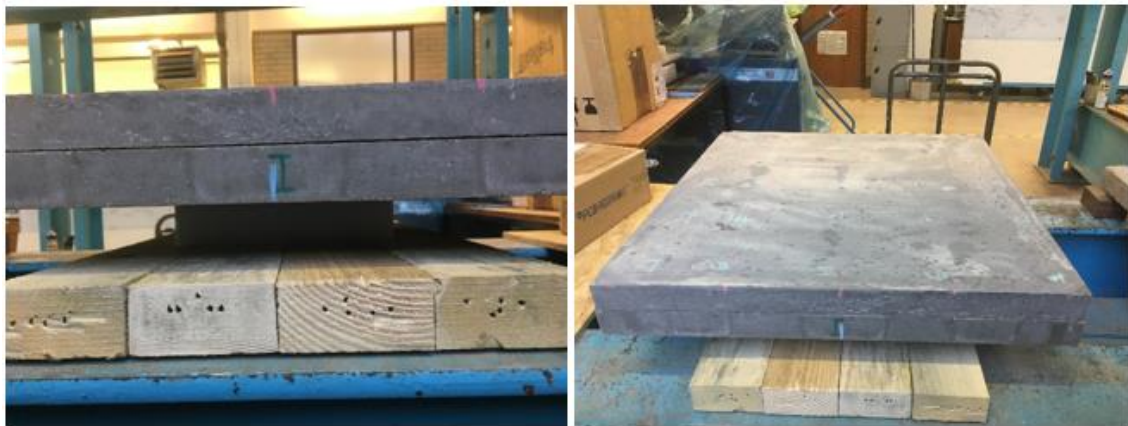
Figure 5-18: Test 02. Two slabs 'fully-debonded', supported on ETHAFOAM 220.
