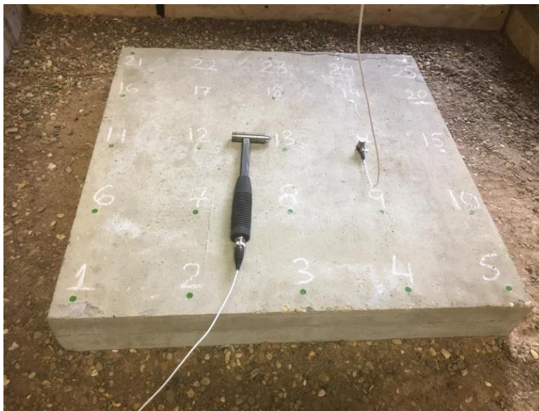
Figure 5-29: Test 05. Two slabs, 'full-debonded' supported on subgrade.
