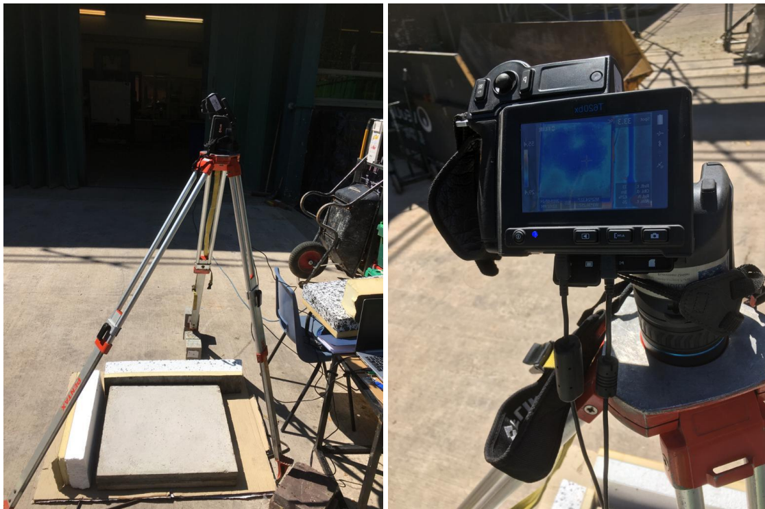
Figure 4-32: Setup of Test 02-IRT. Thermograms recording during the heating phase.
