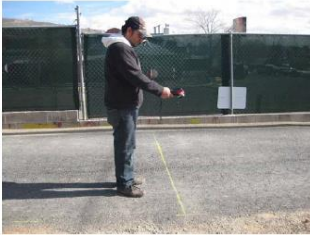
Figure 2-20: Infrared inspection of the HMA pavement (Celaya 2011).
