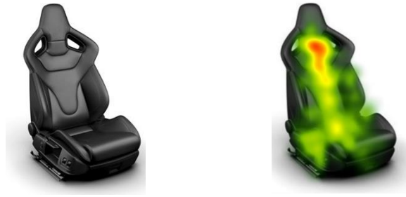
Figure 2: A4 RS4 Sport seat design (left) and cumulative heat map plot (right).
