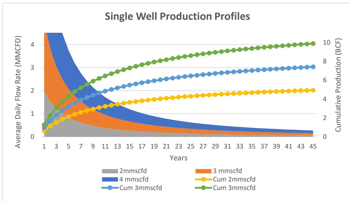
**Figure 5: Production Curves/ Profiles for a Single Lateral Well**
