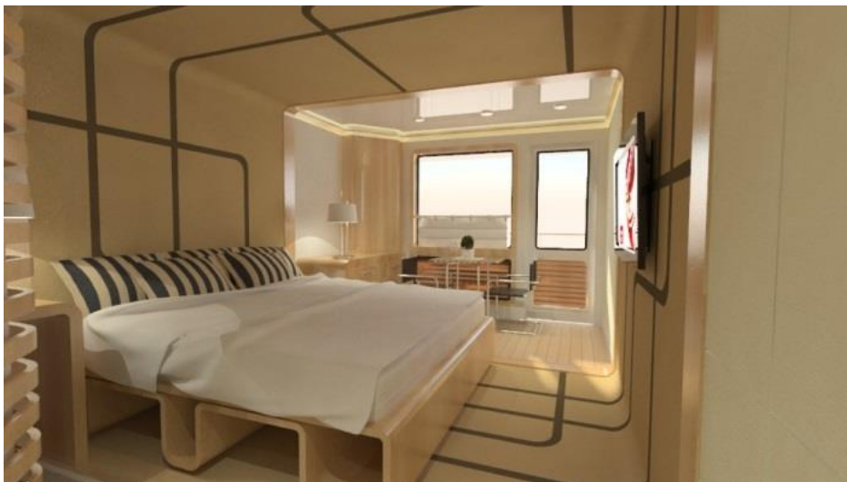
Figure 60: Cabin 3D perspective, looking outboard - with windows featuring a venetian blind mechanism combined with a low-level LED lighting scheme, visually extending the appearance of the glazed area from the floor to the ceiling whilst minimizing the ‘window to wall ratio’
