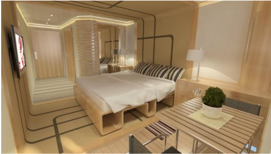
Figure 59: 3D perspective view looking inboard of a cabin - with features allowing natural lighting to permeate deeper into the zone including; higher reflectance flooring nearer the glazing aperture and a bright light color scheme
