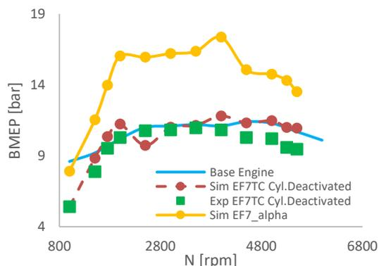
Figure 17. BMEP comparison, EF7 $\alpha$  via base engine
