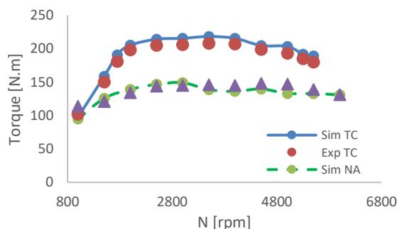
**Figure 11.** Brake torque comparison, EF7TC via EF7NA
