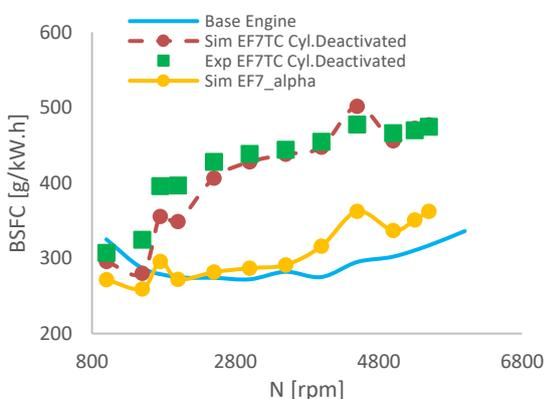
Figure 18. BSFC comparison, EF7 $\alpha$  via base engine
