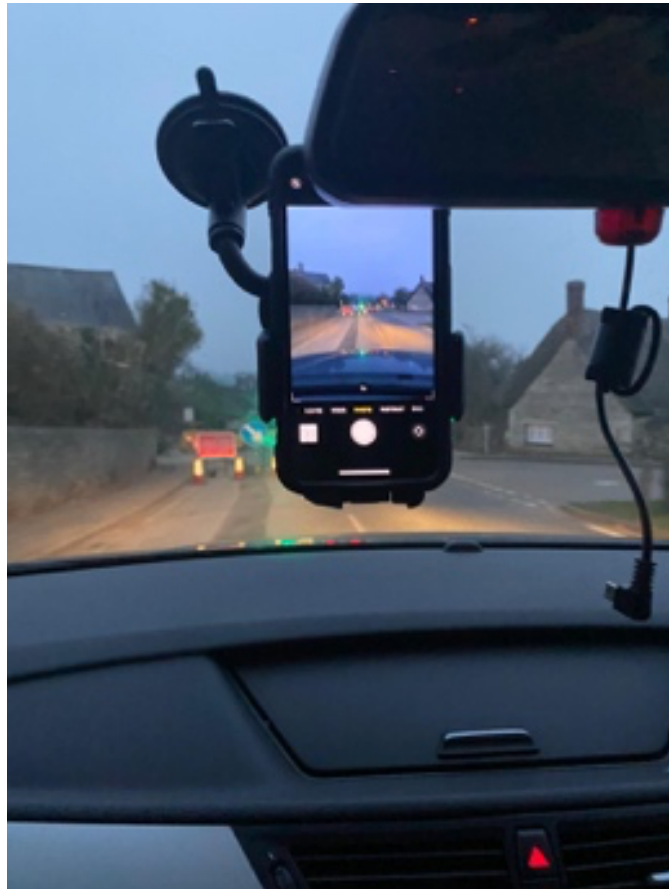
Figure 24: Smartphone placement at the windshield
