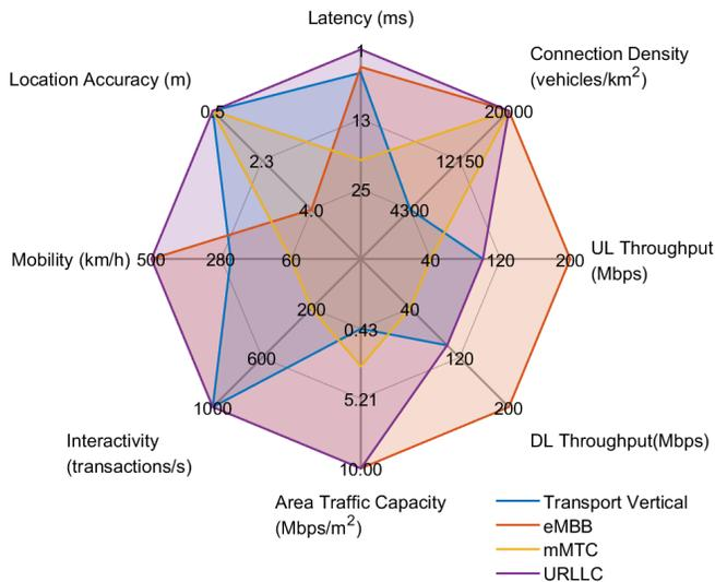
Fig. 3. KPIs of the entire Transport vertical and related 5G service types.
