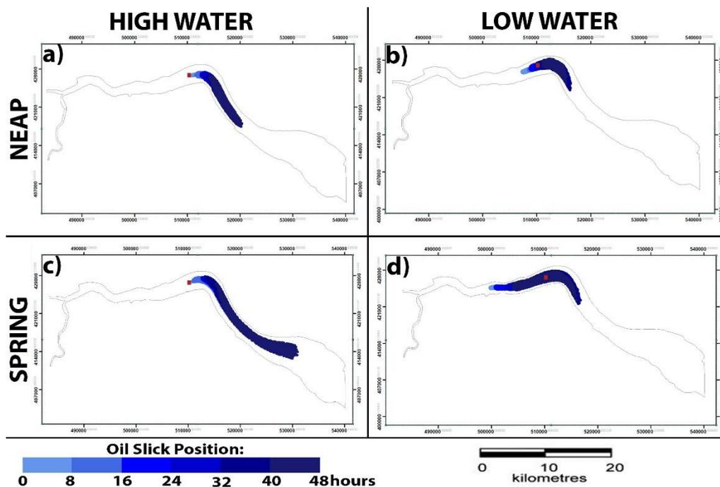
Figure 5: Simulated trajectories of oil released to the Humber Estuary at: a) high water neap tide; b) low water neap tide; c) high water spring tide; and d) low water spring tide. Point of oil release are indicated by red dot.
