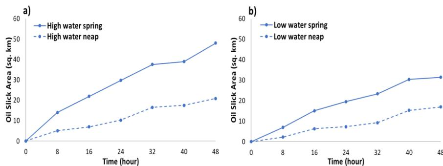
**Figure 6: Area covered by simulated oil slick over time for a spill at: a) high water; and b) low water.**
