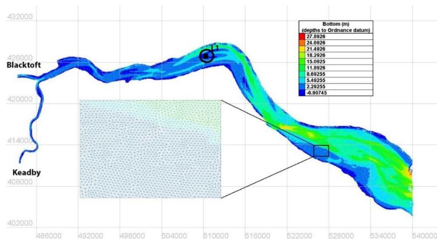
**Figure 2: Bathymetry and computational domain for the Humber Estuary simulations. The release point is indicated by the black dot at 510498; 426777 (coordinates are in OSGB 1936). Inset shows the detail of the computational mesh.**
