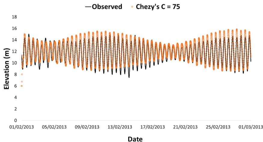
**Figure 4: Observed (line) and simulated (points) free surface elevations at Immingham for the validation period (February 2013).**
