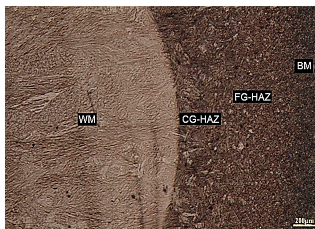
Figure 3. Optical image of weld region in sample No. 5 with a heat input of 2.229 kJ/mm showing WM, HAZ, and base metal.
