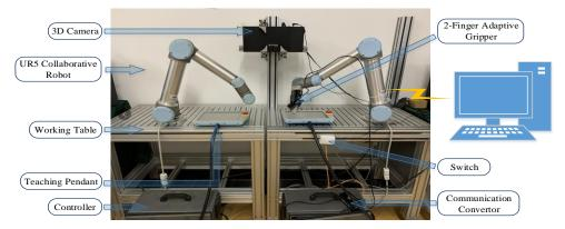
Fig. 9: The experimental platform.
