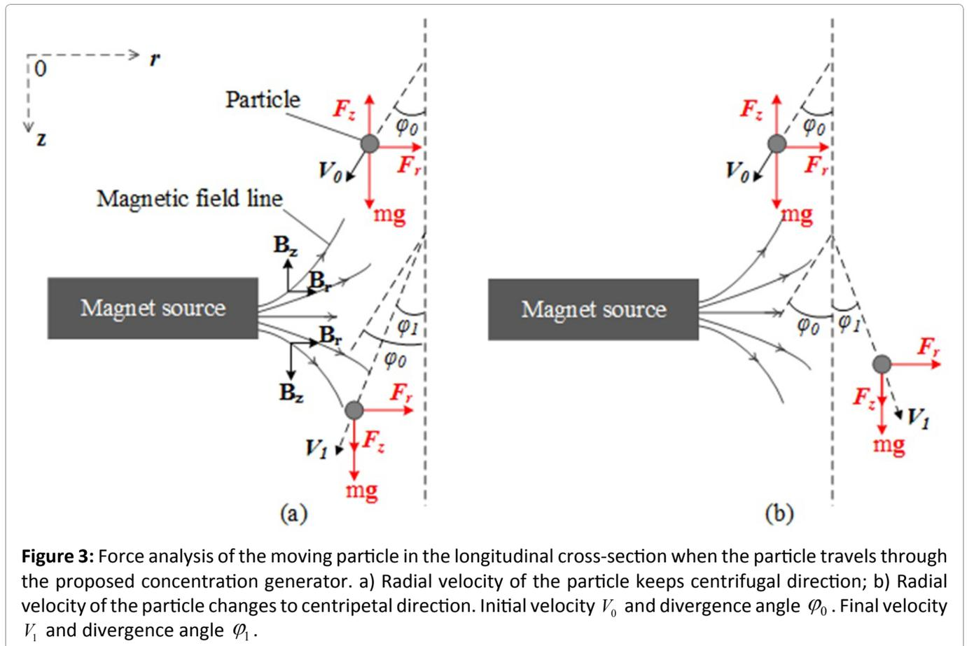
**Figure 3:** Force analysis of the moving particle in the longitudinal cross-section when the particle travels through the proposed concentration generator. a) Radial velocity of the particle keeps centrifugal direction; b) Radial velocity of the particle changes to centripetal direction. Initial velocity  $V_0$  and divergence angle  $\varphi_0$ . Final velocity  $V_1$  and divergence angle  $\varphi_1$ .
