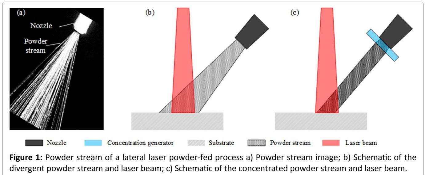
be effectively deposited by a solid-solid surface impact ricochet [2]. Therefore, it is highly desirable to narrow down the diverging powder stream for improving fabrication precision and powder catchment as shown in Figure 1c.
