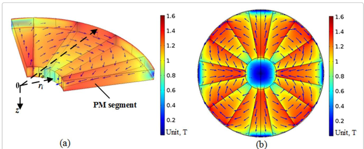
**Figure 5:** Schematic illustration of the proposed magnetic concentration generator with Halbach PM configuration. a) 3D view of the quarter segment and b) Magnetic field intensity norm for the inner region ( $r \leq r_1$ ) of the Halbach PMQs array. Composed by neodymium N52 magnets with residual magnetic intensity  $1.45T$ . The blue arrows represent the magnetic field direction.
