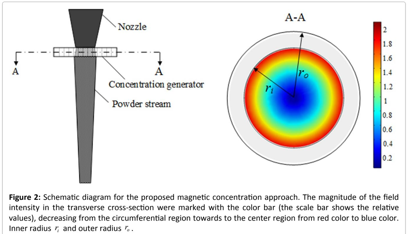
**Figure 2:** Schematic diagram for the proposed magnetic concentration approach. The magnitude of the field intensity in the transverse cross-section were marked with the color bar (the scale bar shows the relative values), decreasing from the circumferential region towards to the center region from red color to blue color. Inner radius  $r_i$  and outer radius  $r_o$ .
