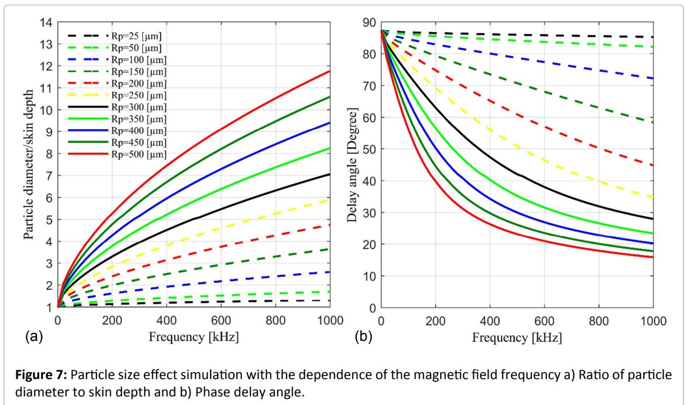
**Figure 7:** Particle size effect simulation with the dependence of the magnetic field frequency a) Ratio of particle diameter to skin depth and b) Phase delay angle.
