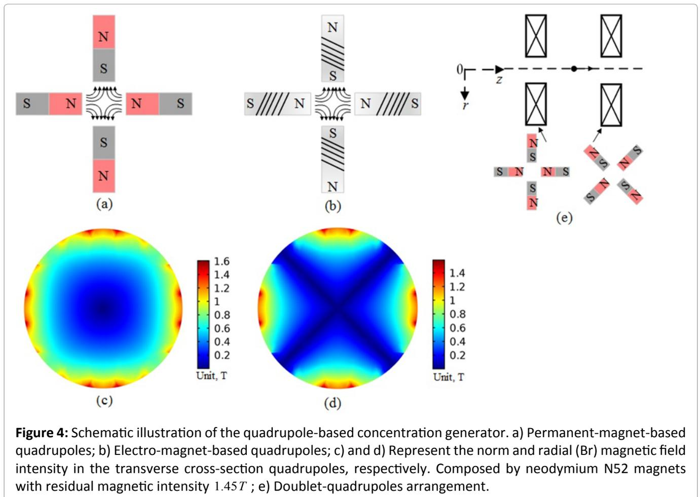
**Figure 4:** Schematic illustration of the quadrupole-based concentration generator. a) Permanent-magnet-based quadrupoles; b) Electro-magnet-based quadrupoles; c) and d) Represent the norm and radial ( $B_r$ ) magnetic field intensity in the transverse cross-section quadrupoles, respectively. Composed by neodymium N52 magnets with residual magnetic intensity  $1.45T$  ; e) Doublet-quadrupoles arrangement.
