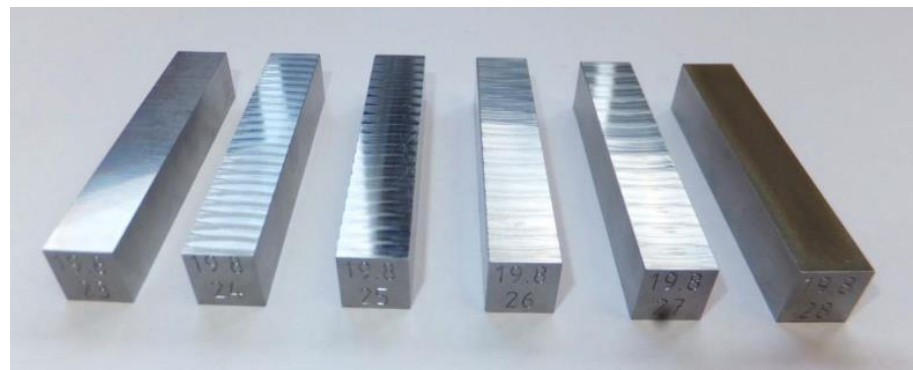
Figure 1. Samples with varying surface roughness conditions used in this study. Specimen 28 (right sample) was obtained by electro-discharge machining (EDM).
