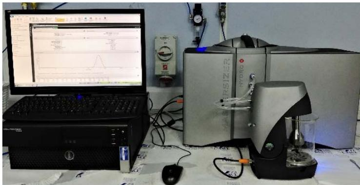
**Figure 3.3** Malvern Panalytical Mastersizer 3000 system used for PSD measurement.
