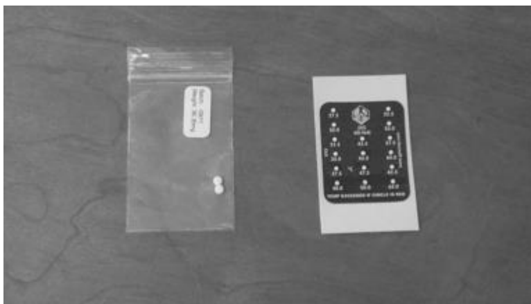
Figure 3. 4: Alanine dosimeter pellets and temperature measurement.
