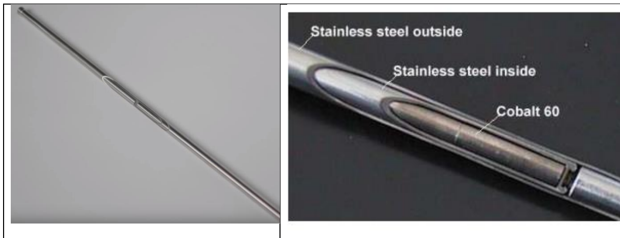
Figure 2. 4: Cobalt-60 metal pellets are double encapsulated in 'pencils' (Sealed Source) (STERIS)
