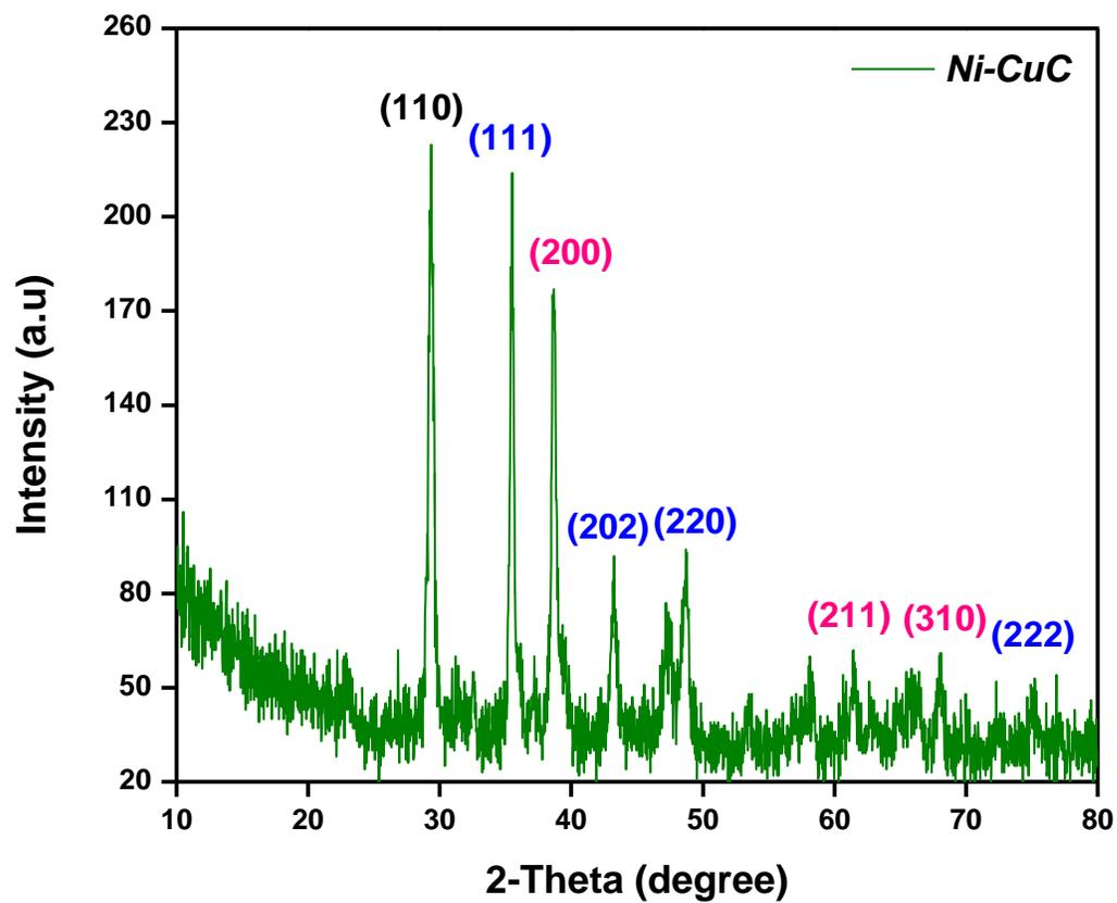
**Fig. 2.** XRD pattern of synthesized Ni-CuC nanocomposites.
