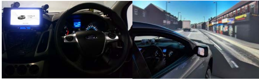
Figure 1. (left) Driver's view of the dashboard and HMI used for activating the automation (right) Driver in-the-loop simulator and its 4.75 meter, 270 degree curved screen.
