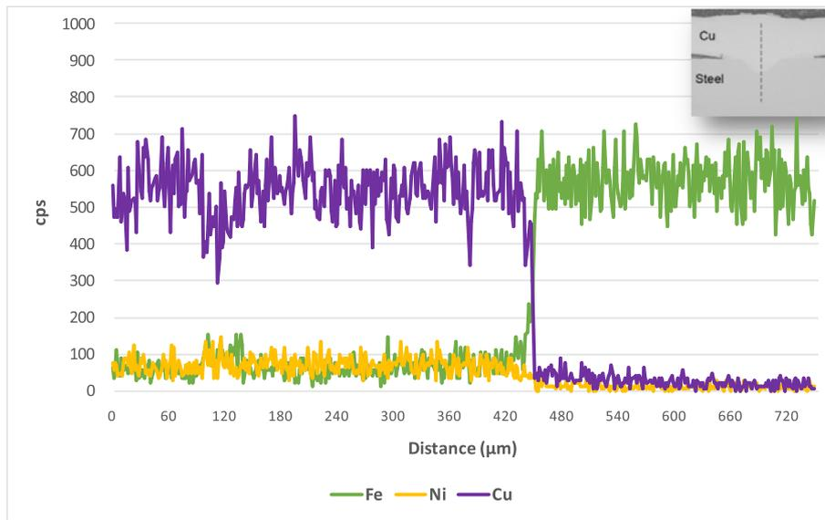
Fig. 6. The EDX line scan inside the weld nugget (see insert) for the sample with a laser power of 1.2 kW.
