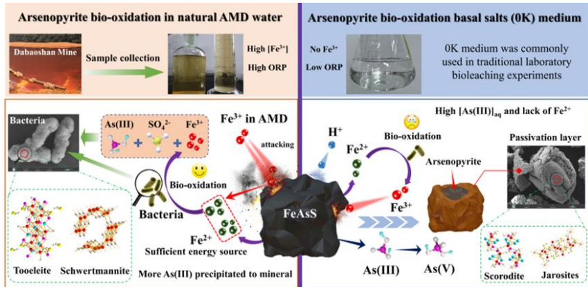
Fig. 8. Schematic diagram of arsenopyrite bio-oxidation and As speciation transformations in AMD (left) and BSM (right).
