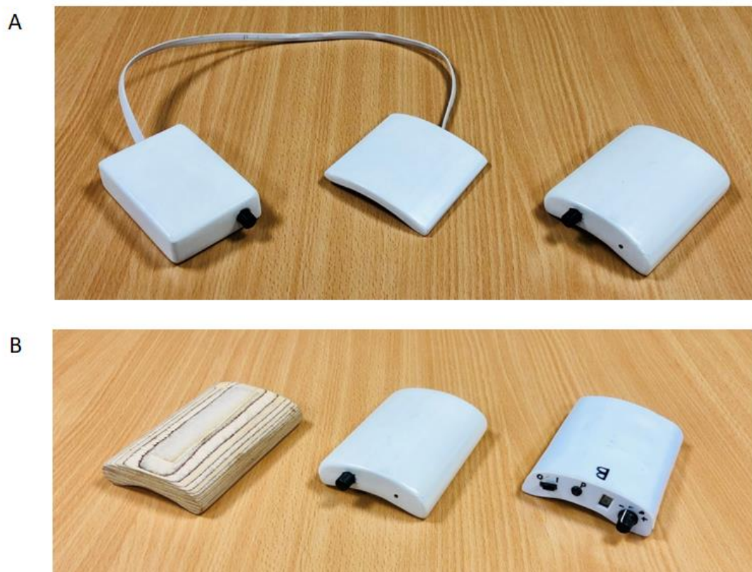
Figure 4. Models created for pre-pandemic usability studies of showing different shapes and forms for the stimulator (A). Models incorporating different control options were later produced (B) [41]
