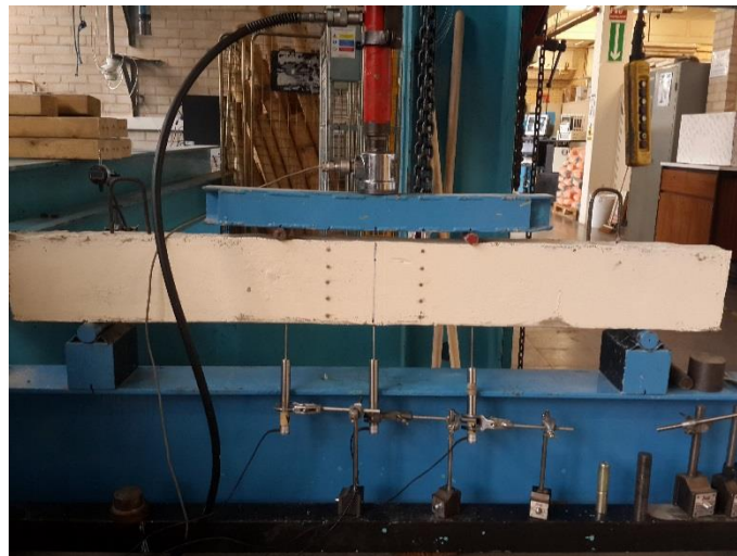
Fig.4 Experimental setup for 4-point loading of beams made from the novel material
