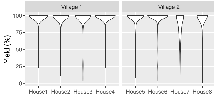
Figure 4.9: PMOG system data yield. The daily yield of the data in % (y-axis) for each household (x-axis). The daily average of yield (%) is above 80% for all PMOG systems installed in the households.
