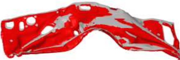
(c) Deformation of the firewall
