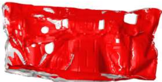
(c) Deformation of the firewall
