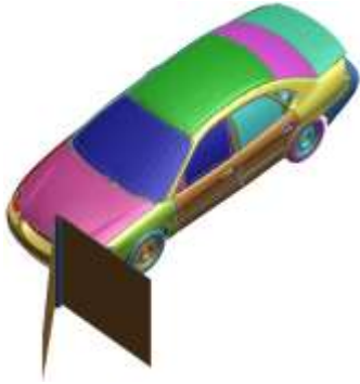
Fig.2. FRB impact simulation model
