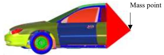
Fig. 6. Schematic diagram of typical simplified schemes
