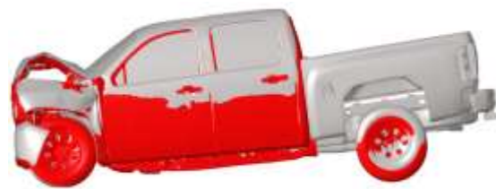
(a) Side view of vehicle deformation
