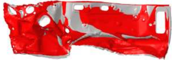
(c) Deformation of firewall
