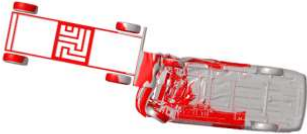
(b) Bottom view of vehicle deformation
