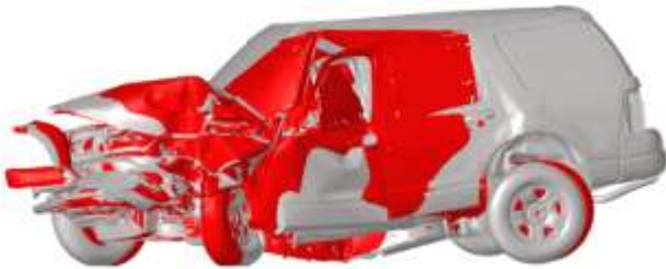
(a) Side view of vehicle deformation
