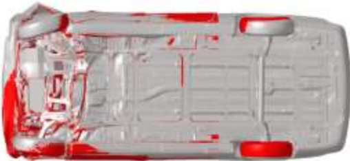
(b) Bottom view of vehicle deformation
