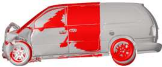
(a) Side view of vehicle deformation
