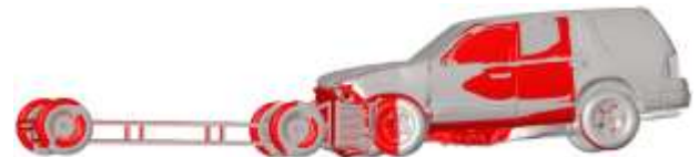
(a) Side view of vehicle deformation
