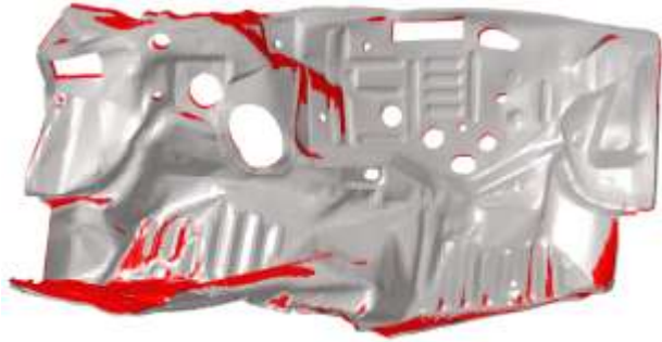
(c) Deformation of the firewall
