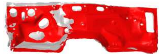
(c) Deformation of the firewall
