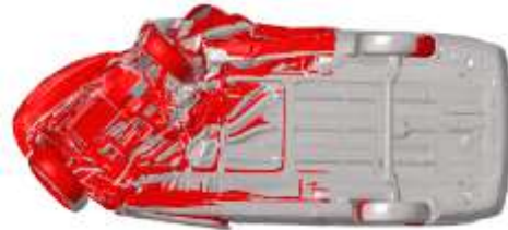
(b) Bottom view of vehicle deformation
