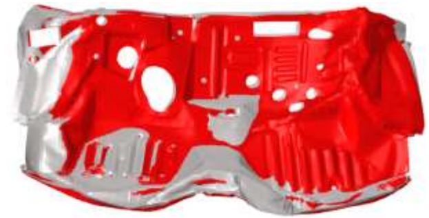
(c) Deformation of firewall
