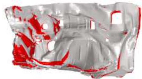
(c) Deformation of firewall
