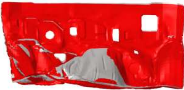
(c) Deformation of the firewall
