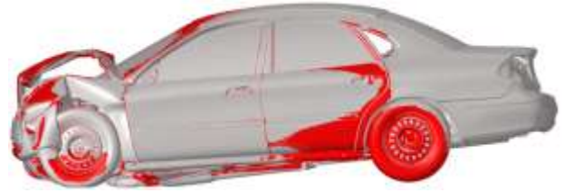
(a) Side view of vehicle deformation
