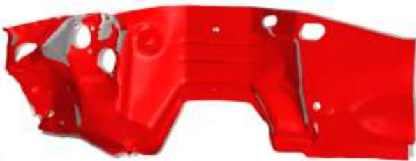
(c) Deformation of firewall
