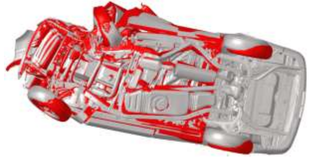
(b) Bottom view of vehicle deformation
