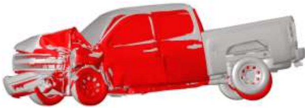
(a) Side view of vehicle deformation
