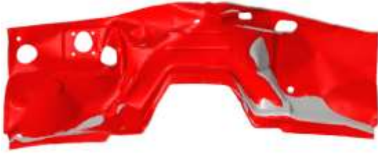
(c) Deformation of the firewall
