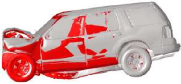
(a) Side view of vehicle deformation
