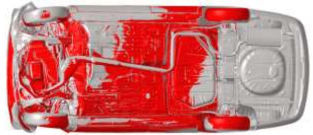
(b) Bottom view of vehicle deformation
