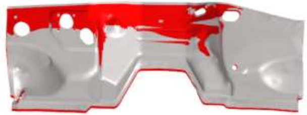
(c) Deformation of firewall
