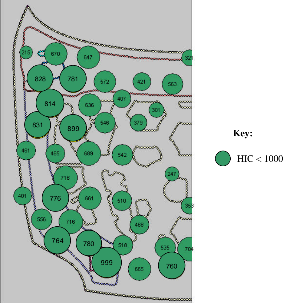
Figure 7. Euro legislation step 1 results for modified bonnets
