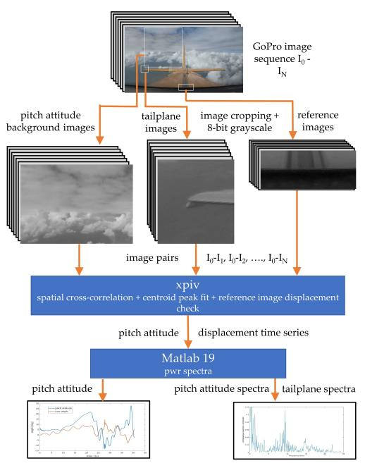
Figure 5. Data processing approach to tailplane, canopy rail reference and pitch attitude estimation.
