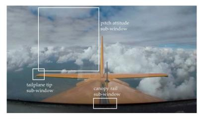
**Figure 4.** Tailplane view in-flight from GoPro camera system. Sub-window images indicate tailplane tip sub-window (201 pixels  $\times$  221 pixels), reference canopy rail (251 pixels  $\times$  101 pixels) and pitch attitude sub-window (910 pixels  $\times$  640 pixels).
