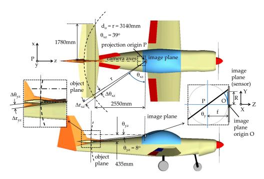
Figure 6. Imaging geometry showing the object and image plane variables.
