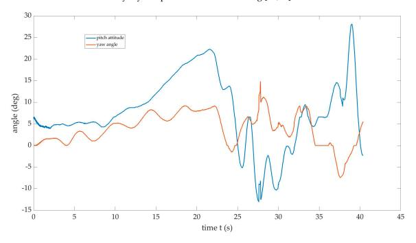
Figure 7. Time series pitch attitude data from GoPro rear view image sequence.
