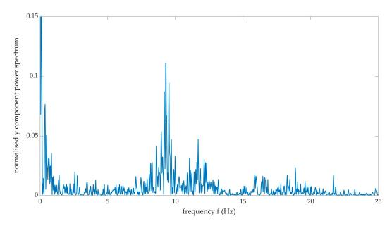
Figure 11. Spectra of GoPro tailplane time series data.
