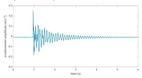
Figure 1. Accelerometer y-axis normalized impulse excitation.
