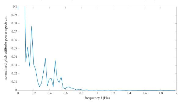
Figure 8. Pitch attitude spectra taken from time series pitch attitude data.
