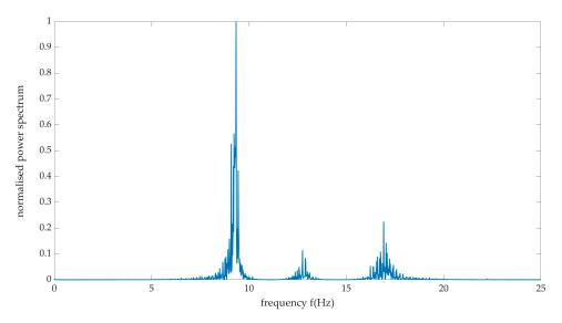
Figure 2. FFT normalized power spectra from y-axes accelerometer output.
