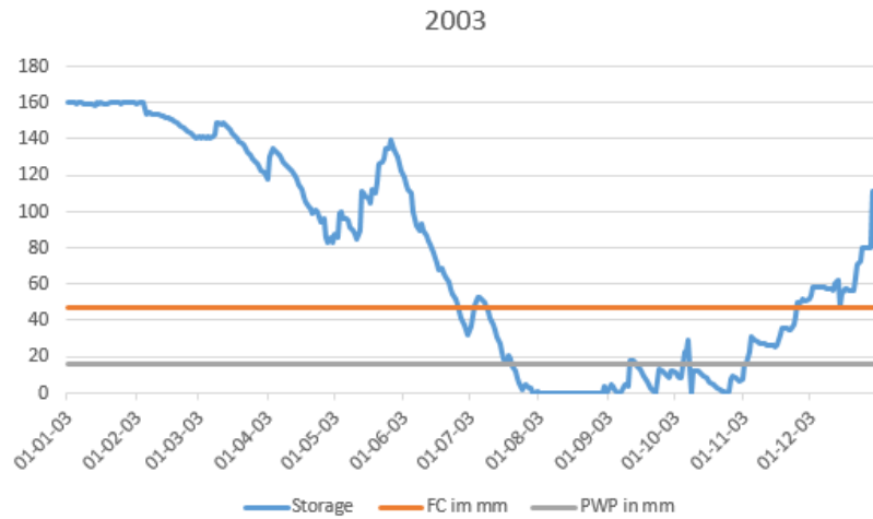
Figure 33: these graphs represent 2003 (dry year) and its response to the change in precipitation values in examining the uncertainty in rainfall data. By change the precipitation values using random high and low range of rain fall in mm in odd months, the graph a moderate change in the substrate (water in soil) moisture content and a change in the liquid water (permavoid) significantly. this significance of responding to change in random values is due to the low rain fall amount in 2003. the X access presents is time in days and the Y access is the moisture content in the “storage” in mm
