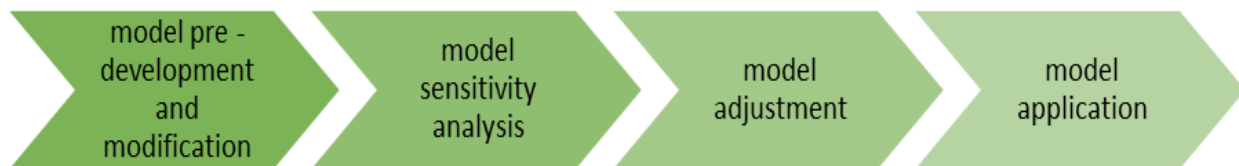
Figure 38: four stages of modification that occurred on the model in order to study the hydrological behavior of green park and managing the moisture content of the system
