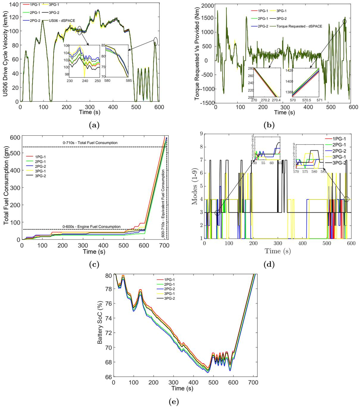
**Figure 4.11:** Real-time SIL results of all five topologies for (a) US06 drive cycle, (b) Torque demand requested vs provided, (c) Total fuel consumption, (d), Modes selection (f) Battery state of charge.
