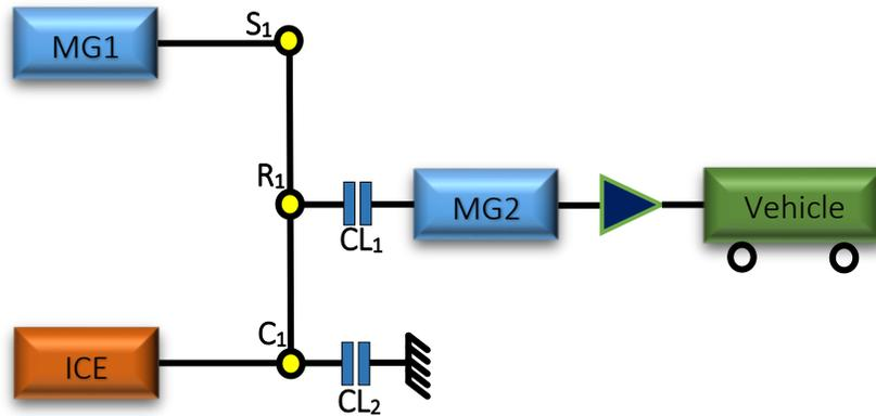
**Figure 2.1:** Schematic diagram of series hybrid electric vehicle, where  $S_1$ ,  $C_1$ , and  $R_1$  are the sun, carrier, and ring gears of 1<sup>st</sup> planetary gear.
