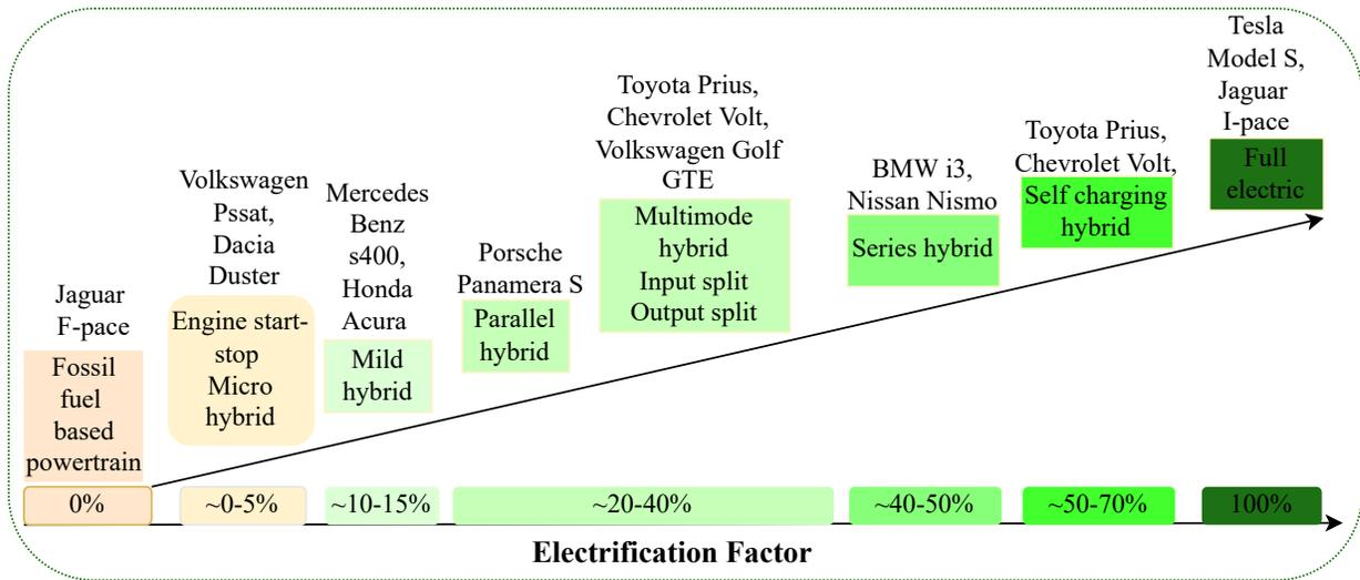
**Figure 1.2:** Classification of powertrains based on electrification factor
