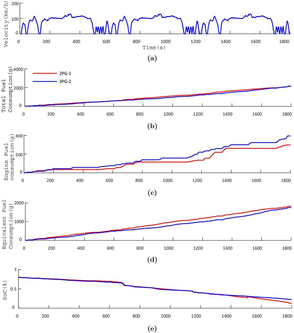
**Figure 3.20:** Fuel consumption over US06 drive cycle for 2PG-1 and 3PG-2 topologies till SoC is below 20% (a) US06 drive cycle, (b) Total fuel consumption, (c) Engine fuel consumption, (d) Equivalent fuel consumption, (e) Battery state of charge.
