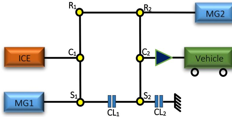
**Figure 2.4:** Schematic diagram of multi-mode hybrid electric vehicle
