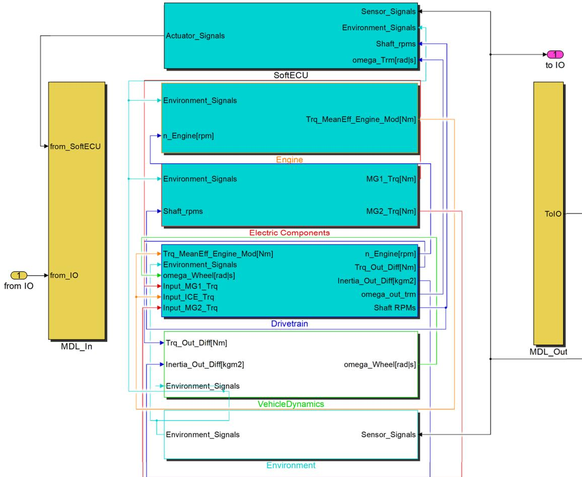
Figure 4.2: First layer layout of developed SIL model
