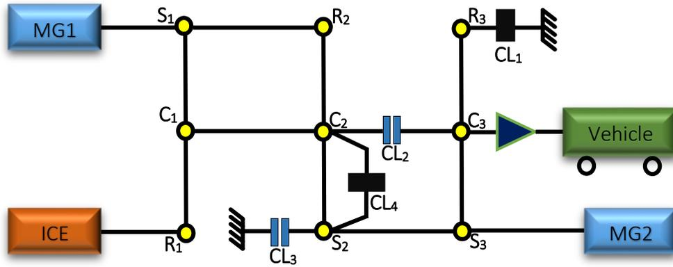
**Figure 2.2:** Schematic diagram of parallel hybrid electric vehicle, where  $S_1$ ,  $C_1$ , and  $R_1$  are the sun, carrier, and ring gears of 1<sup>st</sup> planetary gear,  $S_2$ ,  $C_2$ , and  $R_2$  are the sun, carrier, and ring gears of 2<sup>nd</sup> planetary gear,  $S_3$ ,  $C_3$ , and  $R_3$  are the sun, carrier, and ring gears of 3<sup>rd</sup> planetary gear.
