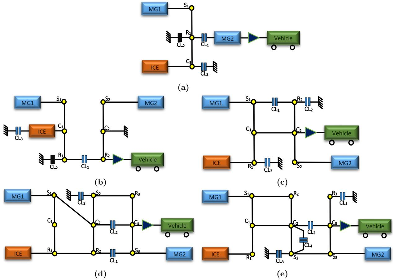
**Figure 3.2:** Different types of topologies used in this study (a) 1PG topology, (b) 2PG-1 topology, (c) 2PG-2 topology, (d) 3PG-1 topology, (e) 3PG-2 topology. The solid black box represents the engaged clutch, while the two thick blue lines represent disengaged clutches.
