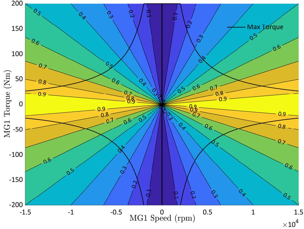
**Figure 3.4:** *The efficiency map of MG [1]*
