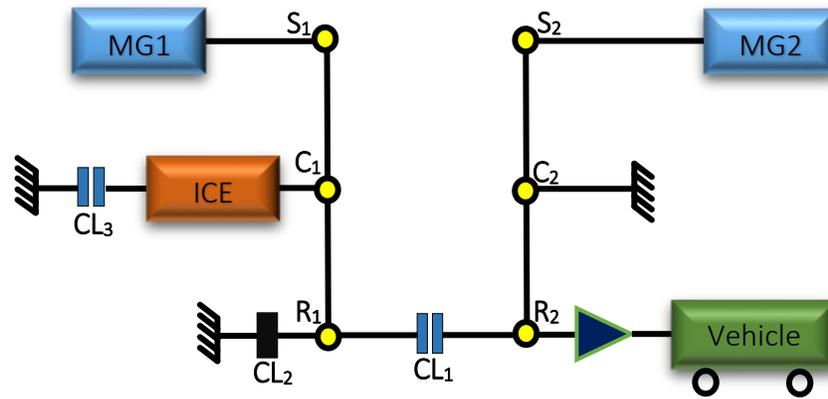
**Figure 2.3:** Schematic diagram of power-split hybrid electric vehicle
