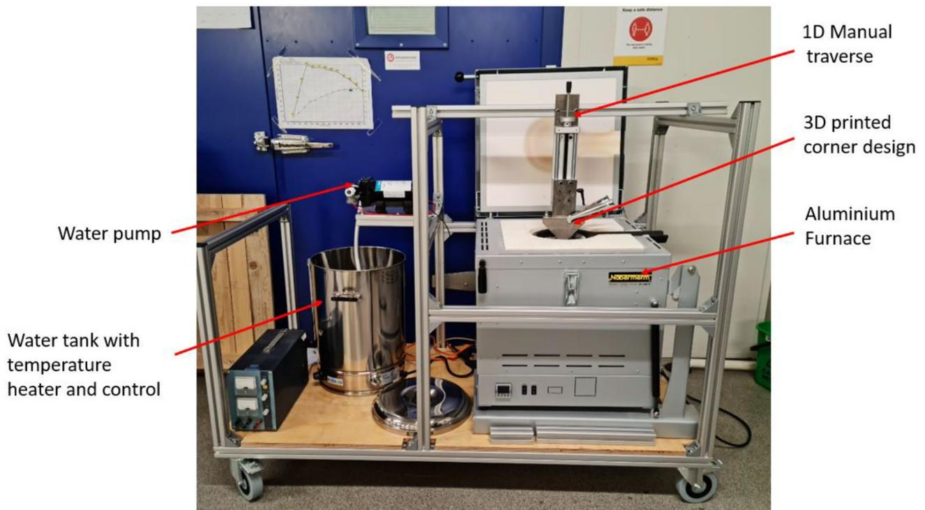
**Fig. 7** Experimental setup for the corner mould design
