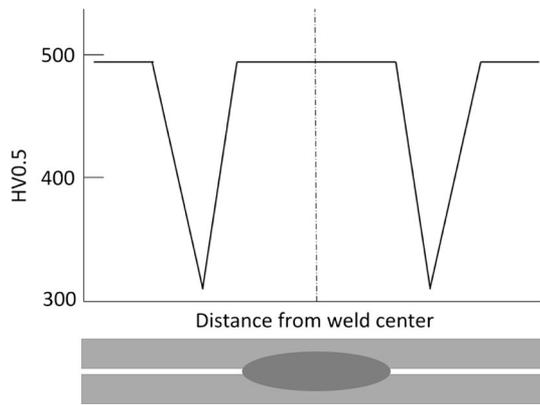
Fig. 1—Hardness profile of press-hardened boron steel spot weld with schematic of RSW work-piece. Adapted from Ref. [8].
