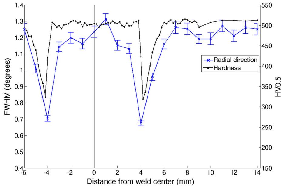
Fig. 16—FWHM of fixed schedule boron steel weld.
