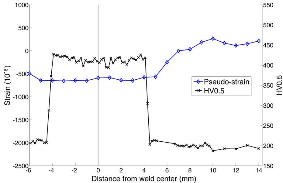
Fig. 12—Variation of pseudo-strain and hardness distribution of DP600 steel RSW welded *via* a fixed schedule.
