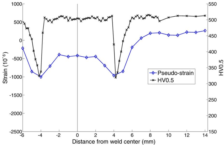
Fig. 10—Variation of pseudo-strain and hardness distribution of boron steel RSW welded *via* a fixed schedule.
