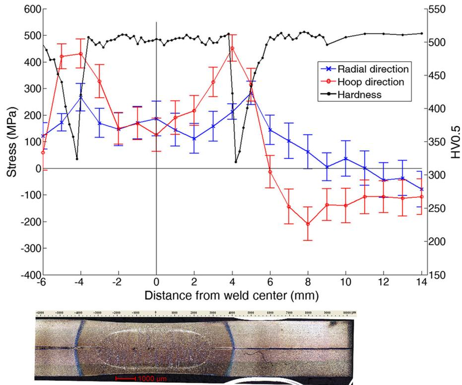
Fig. 13—Calculated residual stress distribution of boron steel RSW welded *via* fixed schedule.
