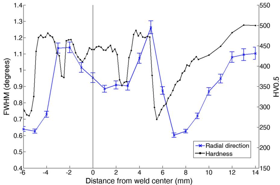
Fig. 17—FWHM of adaptive schedule boron steel weld.
