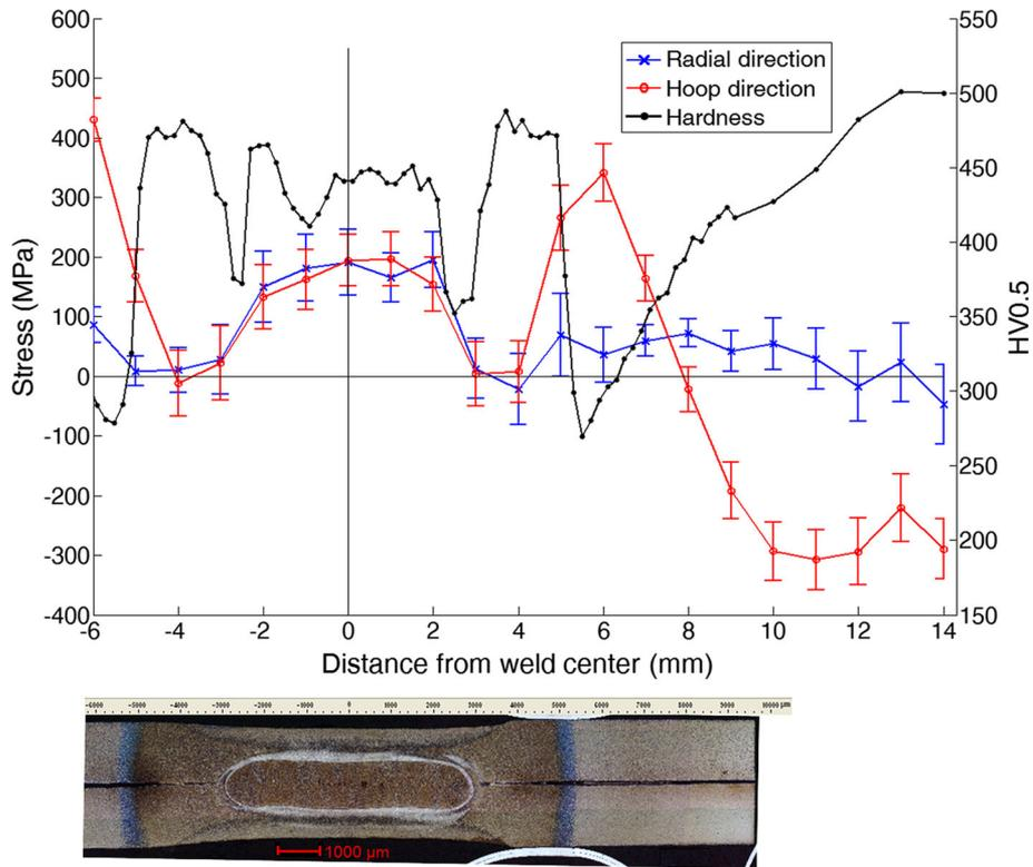
Fig. 14—Calculated residual stress distribution of boron steel RSW welded *via* adaptive schedule.
