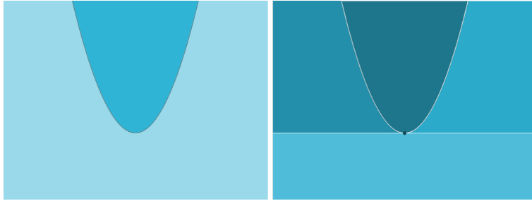
Fig. 1: CADs sign-invariant for x^2 - y in the two possible orderings. The ordering y > x generates the CAD on the left with only three cells (the coloured regions and the curve between). The ordering x > y generates the CAD on the right with nine cells (the four coloured regions along with four line segments and the turning point of the curve).
