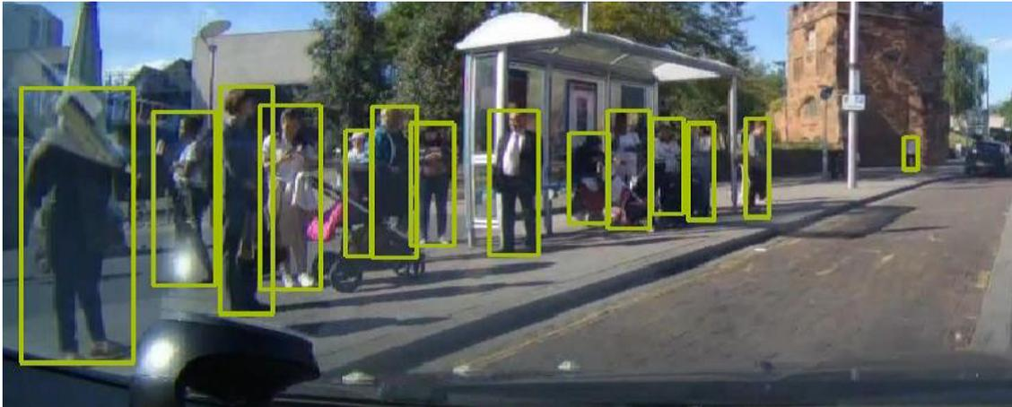
Figure 1: Example of pedestrian detection performed on this project. Each detected object is enclosed by a bounding box with an assigned class and probability.
