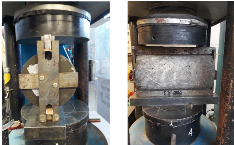
Figure 3.21: Set-up for tensile splitting strength test.
