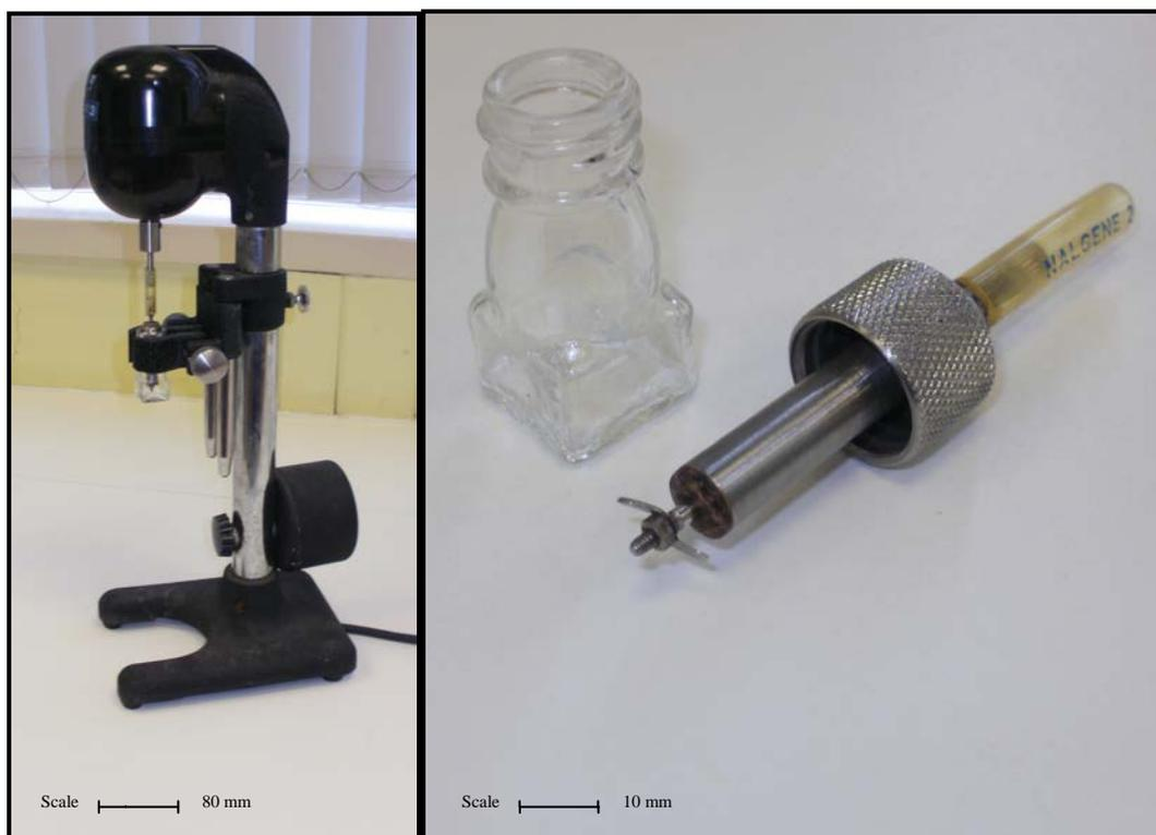
Plate 6.3 - Microhomogeniser, Vial, Blades and Spindle
