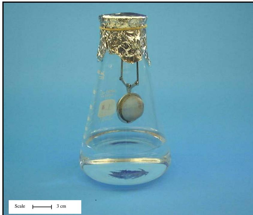
Plate 3.2 - Apparatus Used in the Humidification Treatment.
