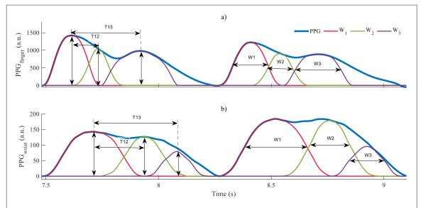
**Figure 9.** An illustration presenting significant differences in the PWD results of synchronized PPG signals from the finger (a) and wrist (b). Here: W1-W3 and T12, T13 are features extracted from decomposed waves  $W_1$ – $W_3$  (see Kontaxis *et al* (2021) for more details about the PWD method).
