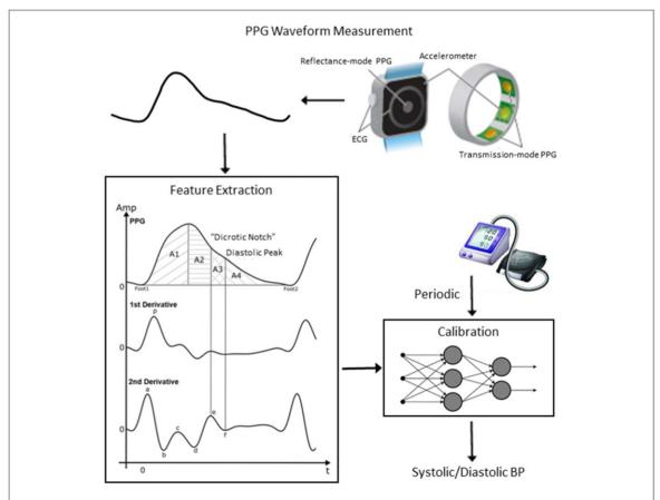
**Figure 28.** Photoplethysmography (PPG) waveform analysis (PWA) for potentially expanding blood pressure (BP) monitoring. Source: Adapted from Mukkamala *et al* (2022b) (CC BY 4.0).
