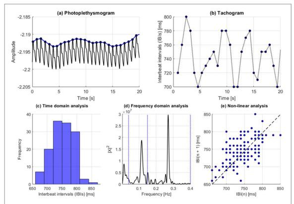
**Figure 7.** Pulse rate variability analysis from photoplethysmograms. Initially, (a) interbeat intervals (IBIs) are detected from the pulsatile signal, and (b) the duration of the intervals is extracted and plotted against time. These IBIs can be summarised using (c) time-domain features, (d) frequency-domain indices, and (e) nonlinear analyses.
