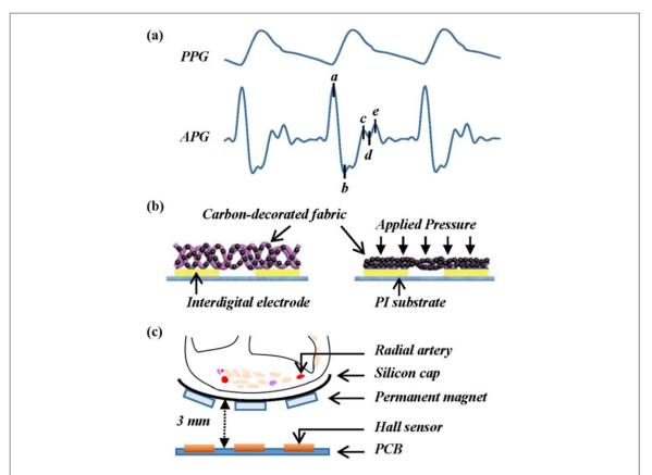
**Figure 32.** Typical processing technique and non-optical sensors used in alternatives of photoplethysmography (PPG). (a) The calculation of the second derivation of PPG to derive the acceleration plethysmography or acceleration PPG (Takazawa *et al* 1998). (b) A piezoresistive sensor for obtaining the impedance PPG (modified from Luo *et al* (2016)). (c) A series of Hall sensors for capturing the magnetic induction plethysmography (modified from Kim *et al* (2018)).
