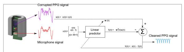
**Figure 5.** Overview of the adaptive noise cancellation of in-ear PPG with a micro-electrical-mechanical systems (MEMs) microphone used as a noise reference to detect minor motion between the sensor and the skin. Source: Adapted from Davies *et al* (2020) (CC BY 4.0).
