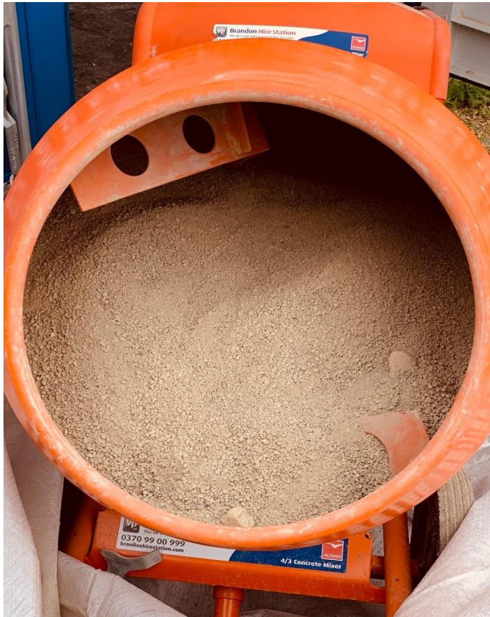
Figure 3.3. Homogenization of Frongoch Mine-Spoils Using a Cement Mixer
